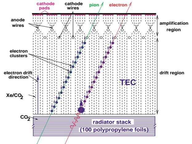
**Fig. 2** T.R.D. principle.
