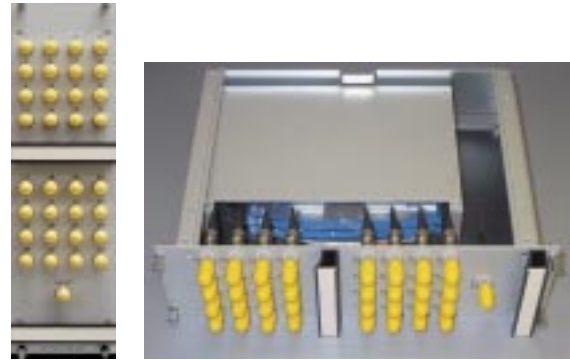
Figure 10: Cassette-mounted 1x32 singlemode tree coupler
