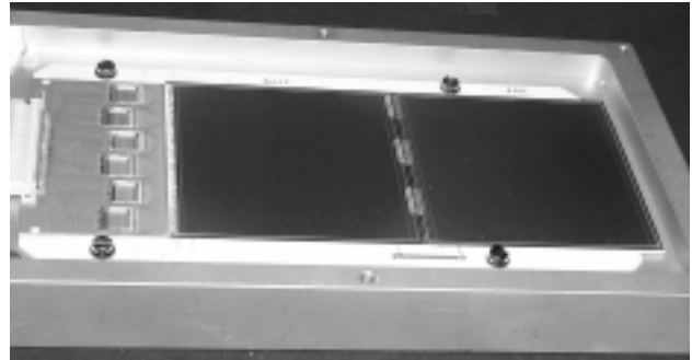
Figure 7: Photograph of a 13-cm module with 6 SCTA128HC chips.
