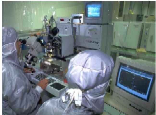
Fig 5: Automatic wire bonding equipment
