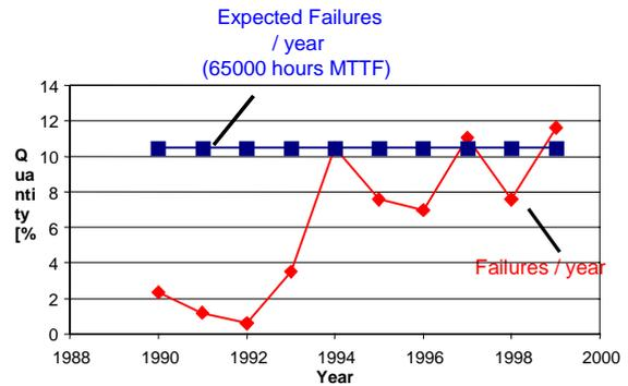
Figure 17. Failure rate of the DELPHI Fastbus power supplies
