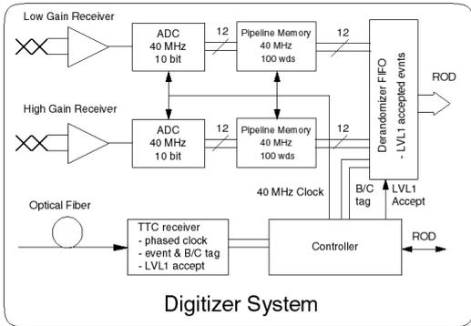
Figure 7. Tiles calorimeter read-out electronics
