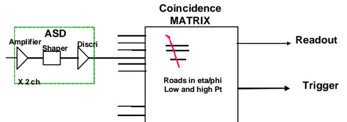
Figure 9. The RPC read-out electronics
