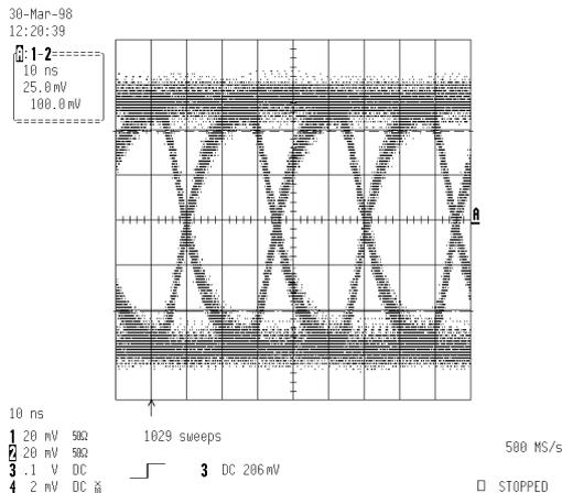
Figure 12. Eye pattern of a 100m 40MHz LVDS copper link after cable compensation.
