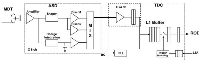
Figure 8. The MDT read-out electronics
