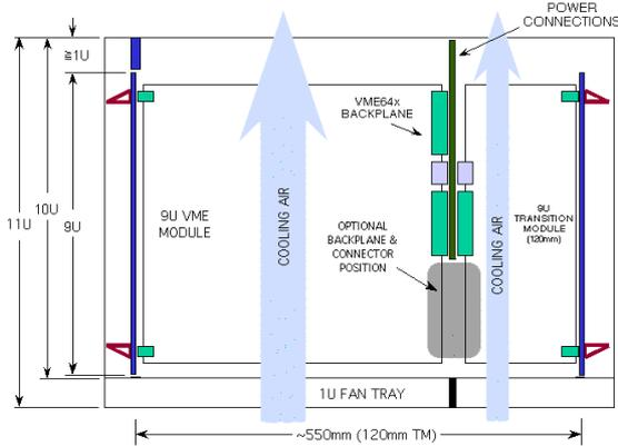
Figure 16. Possible crate lay-out
