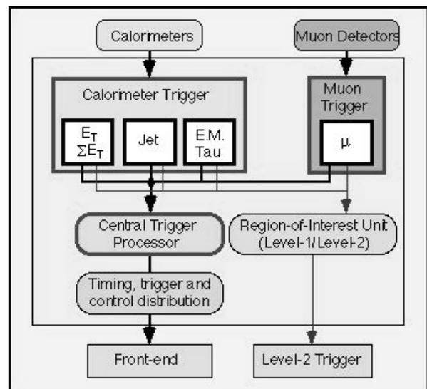
Figure 2. The level-1 trigger system.
