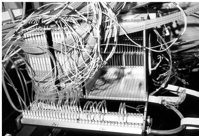
Figure 6. Liquid Argon front-end crate with its cooling tubes
