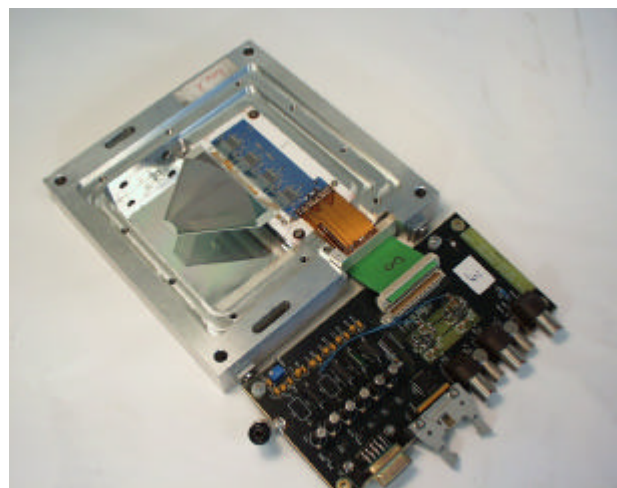
Figure 15: Vertex detector hybrid prototype
