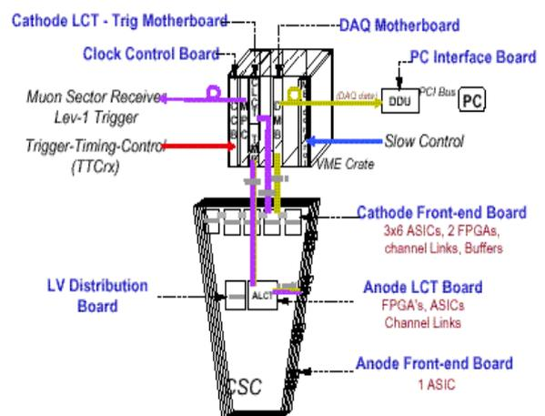
Figure 4 : Muon endcap on-detector electronics
