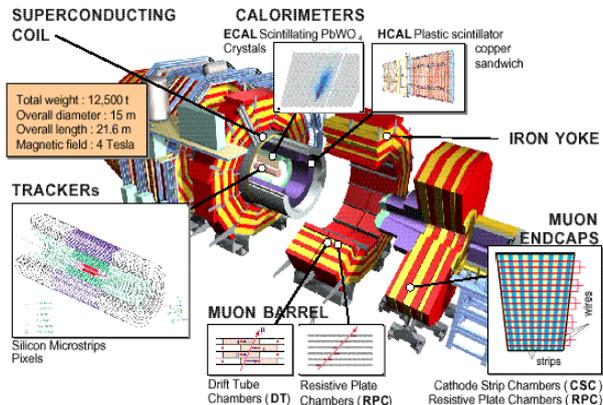
Figure 1: CMS structure and detector technologies.
