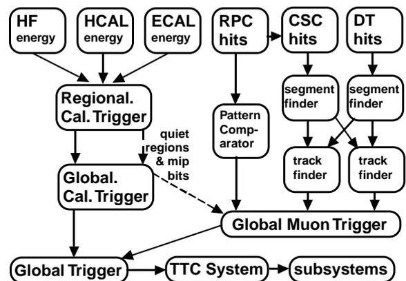
Figure 6: Schematic layout of Level 1 trigger system
