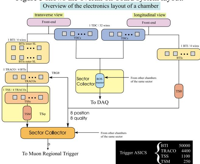
Figure 5: Muon barrel drift tubes on-detector scheme.
