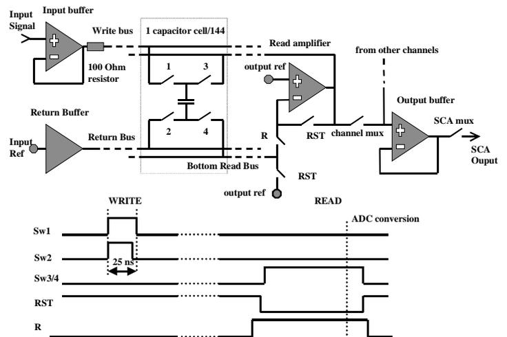
Fig. 4: channel block diagram
