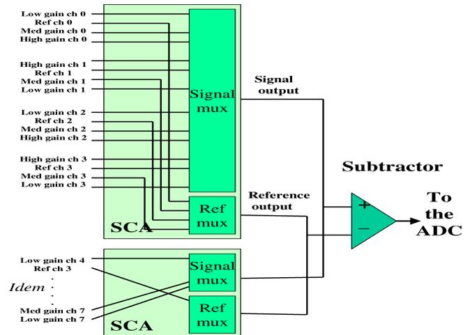
Fig. 2 : output cabling for 8 SCA channels
