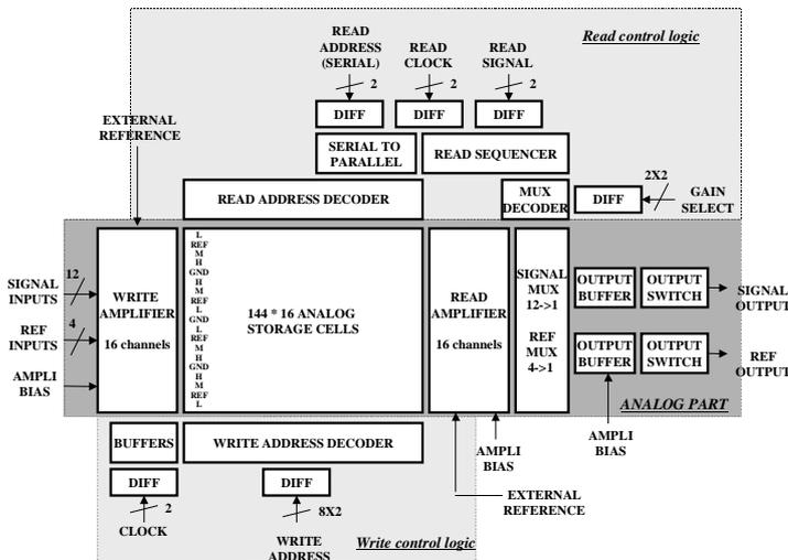
Fig. 3 : analog memory architecture.
