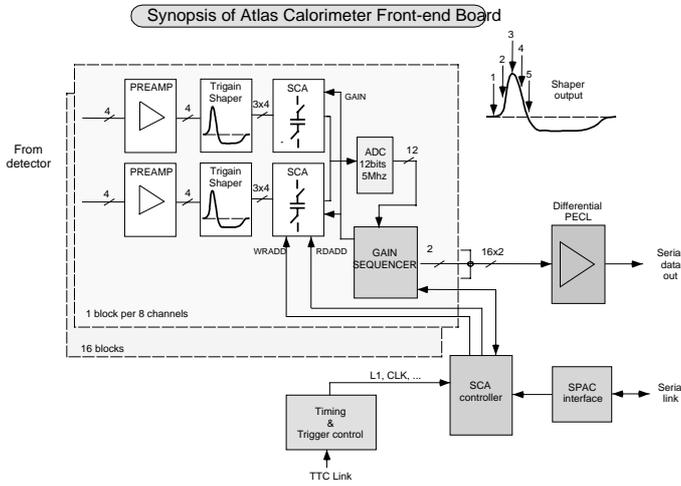
Fig. 1 : block diagram of the *Front-end board*
