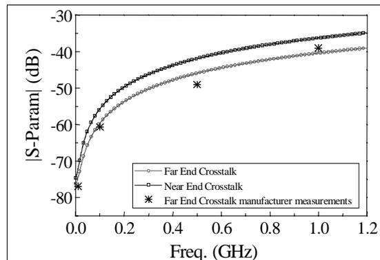
Figure 10: Near-end ( $|S_{21}|$ ) and far-end ( $|S_{24}|$ ) crosstalk
