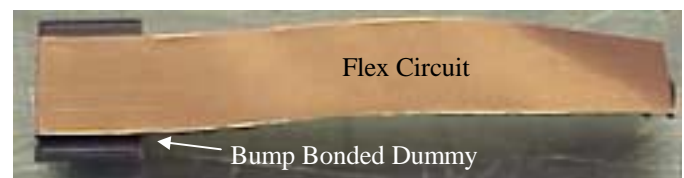
Figure 9: Dummy Bump Bond Structure
