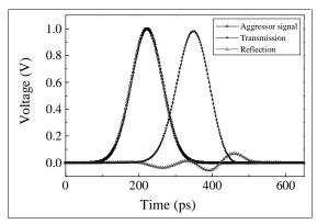
Figure 7: Time-domain connector transmission results.
