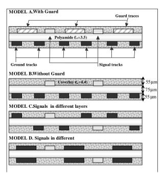
Figure 4: Different signal-ground track configurations.
