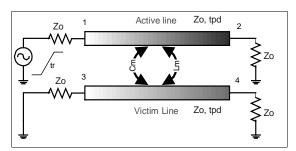
Figure 1: Crosstalk scenario.  $C_m$  models the capacitive crosstalk;  $L_m$  models the inductive one.
