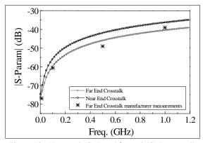
Figure 10: Near-end ( $|S_{21}|$ ) and far-end ( $|S_{24}|$ ) crosstalk
