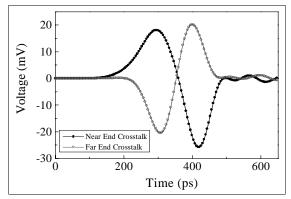
Figure 8: Near-end (port 1) and far-end (port 4) crosstalk
