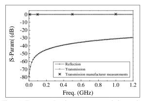
Figure 9: Frequency-domain connector transmission results.
