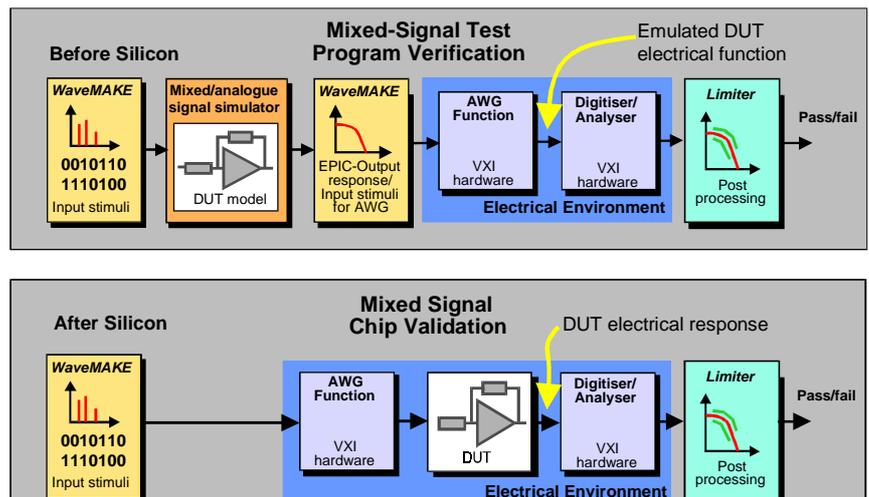
Fig. 11: Illustration of principles in VirtualSTIMULI. In the upper picture, simulated signals are used to generate electrical stimuli for verifying the test setup. In the lower picture, the actual chip is being tested using the hardware modules that were earlier used for test program
