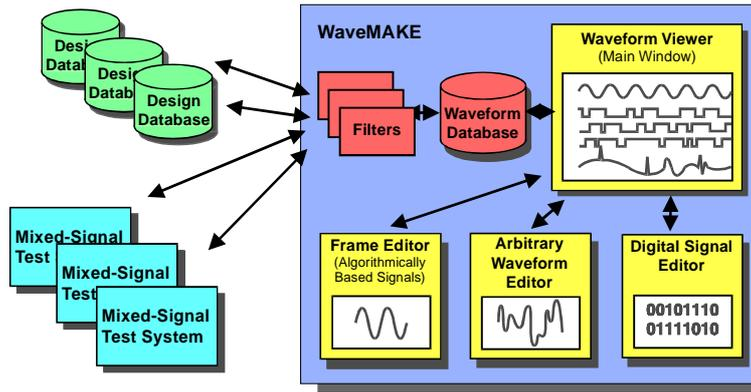
Fig. 8: The WaveMAKE waveform editor and viewer can be used to include all analogue and digital signals in a test. Signals may be transferred from a design database and after integration downloaded to the tester.
