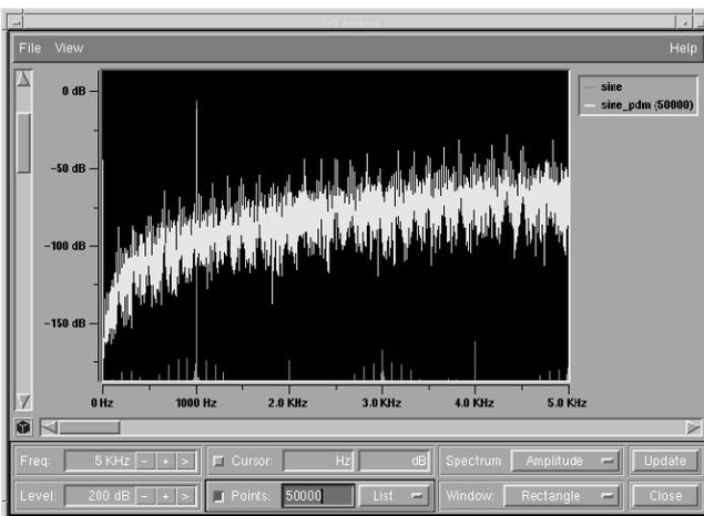
Fig. 9: WaveMAKE easily handles conversions between domains, here analog and digitised PDM signals. The FFT can be invoked on the analog as well as the digitised version of the signal.
