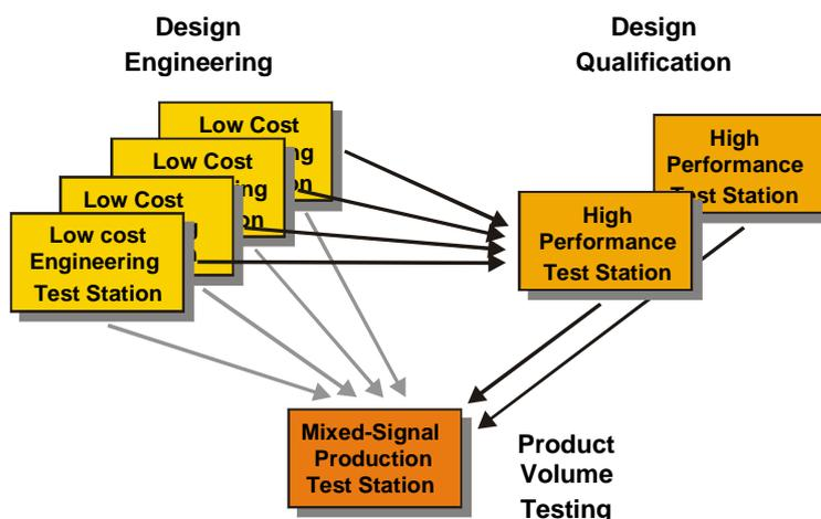
Fig. 2: The 3 lines of mixed-signal test system categories in the scalable solution. The software architecture offers the same look-and-feel at all three levels.
