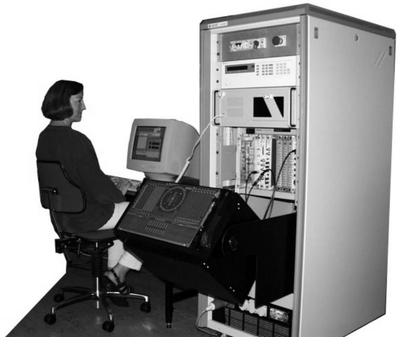
Fig. 5: The production version, Charlie, of the scalable range of test system solutions has separate test head that
