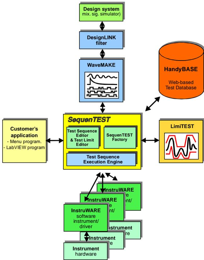
Fig. 7: Software tools of the IntegraTEST scalable test environment consists of test sequencer, limiter functions, waveform editor/viewer, instrument subsystems, test database, etc.
