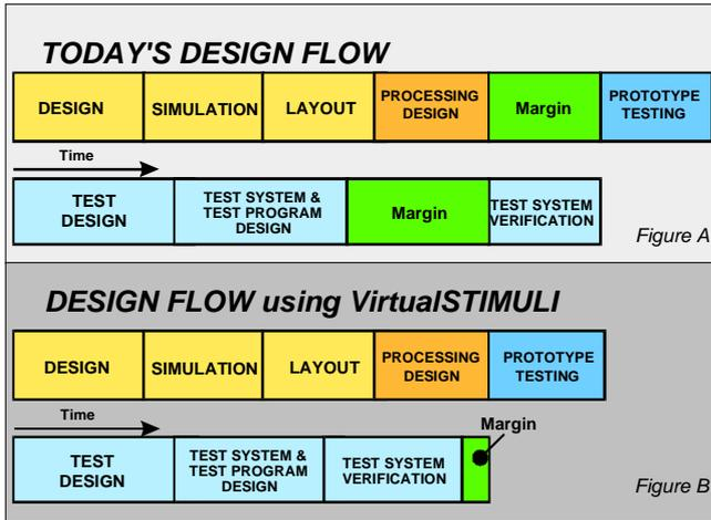
Fig. 10: Today's design flow of mixed-signal can be optimised, if concurrent test generation can take place before actual silicon exists.
