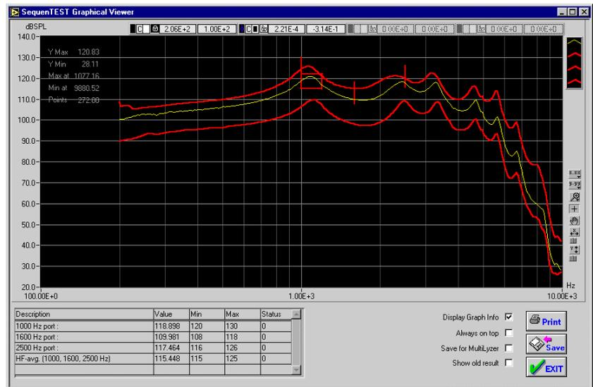
Fig. 6: An example of a tunnel limiter applied to an analog signal. Below the view graph is a table displaying user defines key parameters. All results or subsets thereof can be logged to the test database.
