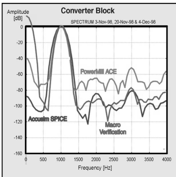
Fig. 12: Verification of simulated results for an advanced mixed-signal macro block (Spice and functional simulation) versus actual macro verification of the silicon.
