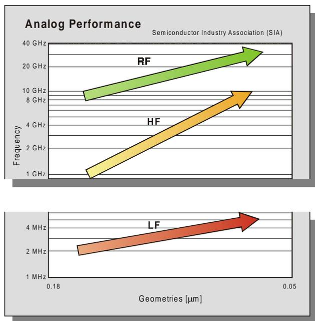
Fig. 1: The performance of CMOS analog is closing in on bipolar performance up to year 2012.
