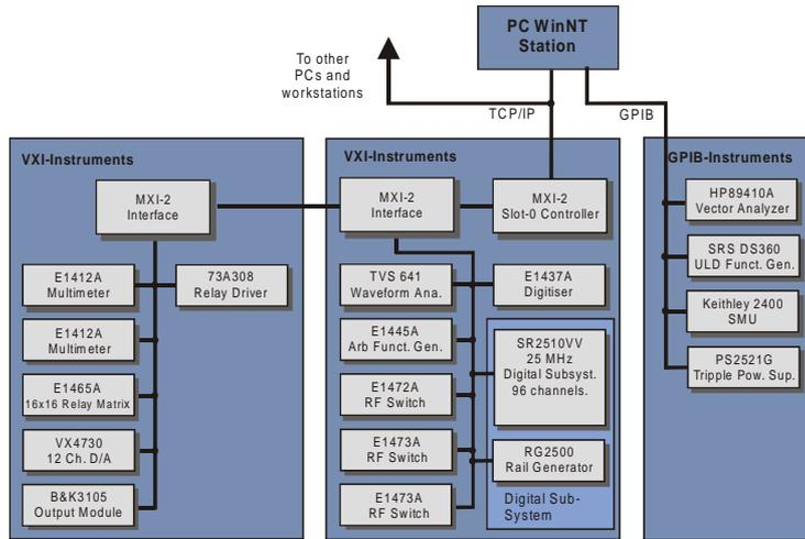
Fig. 4: A typical example of instruments in a high performance Bravo test station. Most instruments are contained in two VXI racks, but some GPIB-bus controlled instruments are employed as well.
