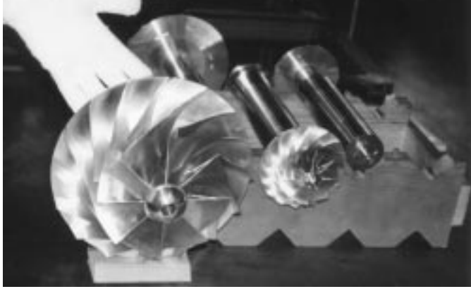
Figure 6: Impellers of cold compressors for the first 2.4 kW @ 1.8 K refrigeration unit
