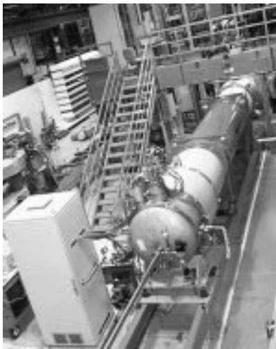
Figure 4: First pre-series superconducting magnets under test. a) Main dipole at CERN; b) Low- \beta quadrupole at Fermilab
