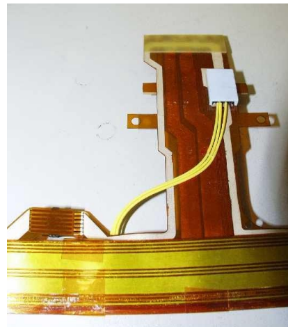
Figure 3 Opto-flex and Aluminium low mass cables with three fibres in furcation tubing.
