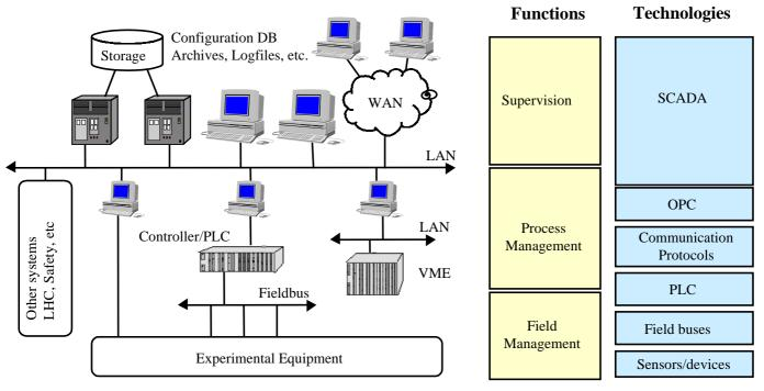
Figure 1: Example LHCb Architecture
